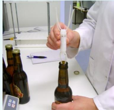
Spider cap is used inside the bottle to keep the logger centered
